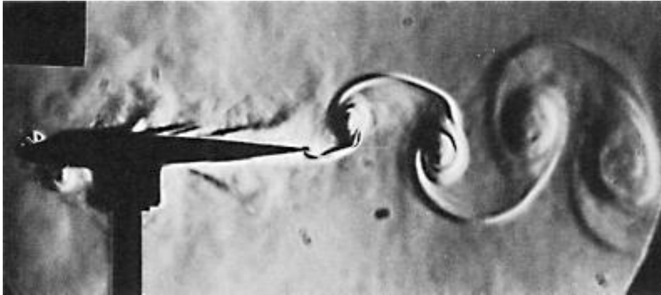
Fig.16.12 Flow at bottom dead point of vertically vibrating wing (Schlieren method) in air, flow velocity 5 m/s, chord length 100 mm, Re \approx 3 \times 10^4 , vibration frequency 90 Hz, single amplitude 4 mm
