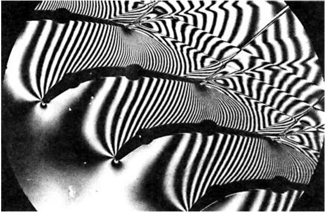
Fig.16.14 Equidensity interference fringe photograph of driven blade on low-pressure stage in steam turbine (Mach-Zehnder interferometer method) in air, inlet Mach number 0.275, outlet Mach number 2.123, pitch 20 mm
